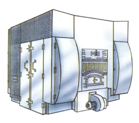
The air heater is capable of a thermal efficiency of 84%. The burnt gases after combustion passes through a series of tube banks which is a Three pass type. and is exhausted to the atmosphere through an under ground flue using an induced draft fan of the centrifugal type. The heater can be arranged for Wood, coal or oil firing.
